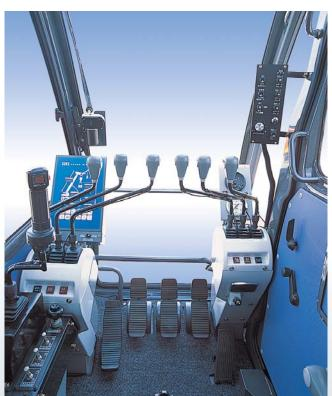
Boom extension/retraction, hoisting/lowering can be operated separating from other movement. Since the capability of simultaneous operations is available for the extension/retraction, hoisting/lowering, the positions of front attachments can be set up easily and precisely. Boom hoisting can be operated both control lever and left foot pedal, complicated multiple operation can be possible easily.
